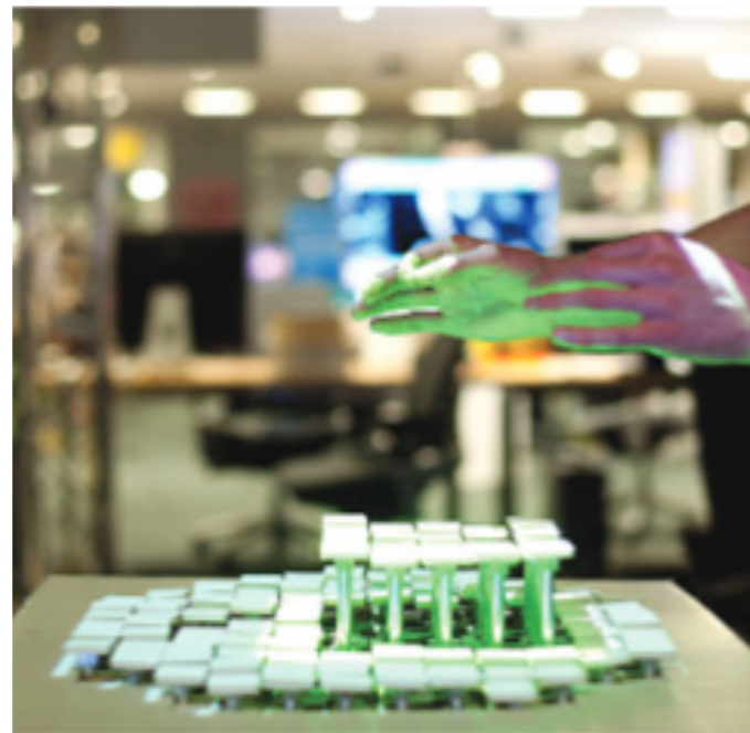
Figure 27: A physical shape that can deform with integrated sensors (Yao et al., 2013)
