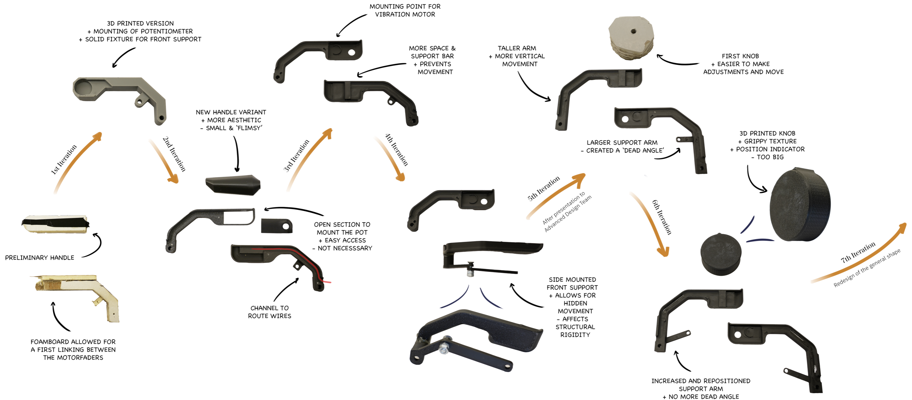
Figure 74: Handle process - pt.1
