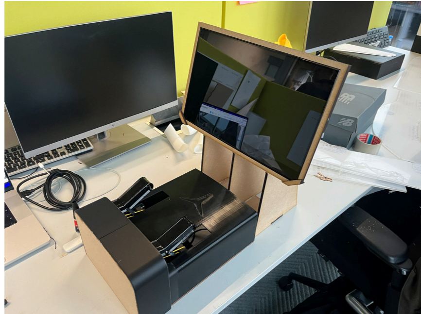
Figure 69: Laser-cut monitor housing/hyperscreen holder attached to interface enclosure
