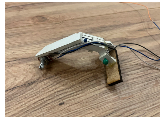
Figure 56: First handle with integrated potmeter
