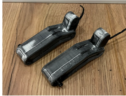
Figure 66: 3D prints with filler and sanded
