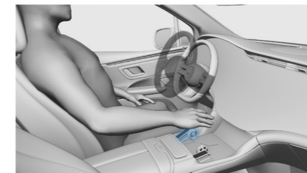
2. Once the automated driving takes over, the driver can activate 'Glide'. This retracts the steering wheel and moves the tangible interface into the base position.
