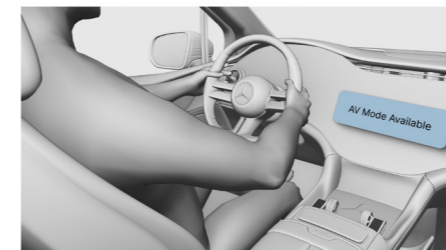
1. The driver drives the vehicle until the automated driving can take over and a takeover is initiated.
