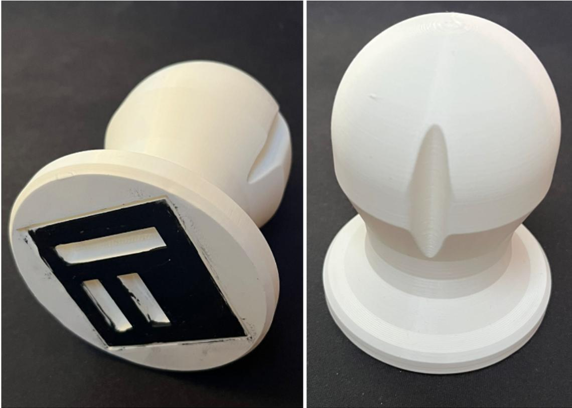
Fig. 3. Image of the 3D printed controller with the CV marker on the bottom
