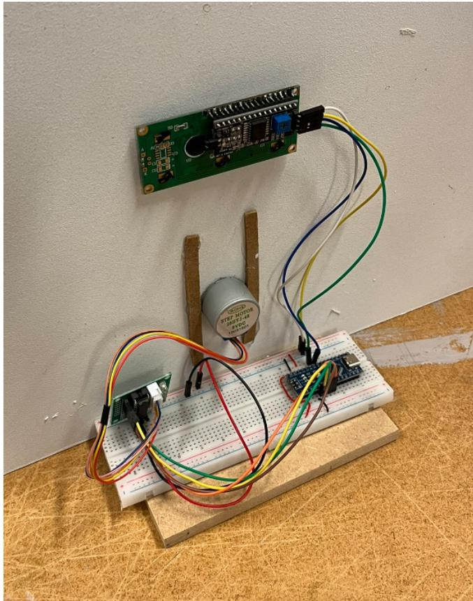
Fig. 2. Image of the circuitry. (The lamp is not connected but would simply be attached to pin 9)
