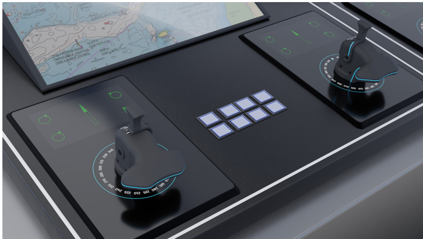
Figure 130: Final Concept rendered in a tugboat bridge mounted onto the Smart-Ship hardware.
