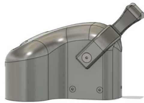
Figure 93: Form concept control unit with throttle engaged at 45 degree
